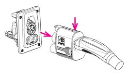
2. Pull the plug out of the adapter with pressing the NACS Unlock Button on the side of the adapter.
