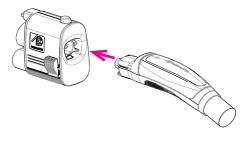
2. Align the adapter plug with vehicle's charge port, and fully insert the plug into the port.
