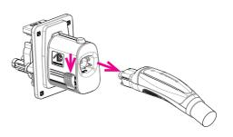
2. Remove the adapter from the vehicle with pressing the CCS1 Unlock Button on the top of the adapter.
